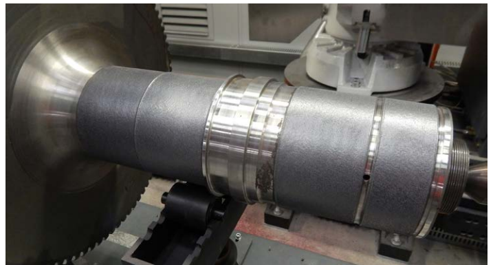
Repair of shafts with iron-based alloys
