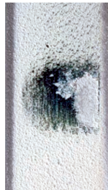
Mixed coating rupture and blade material transfer
