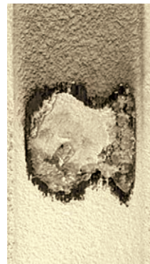
Heavy coating rupture after initial blade material transfer
