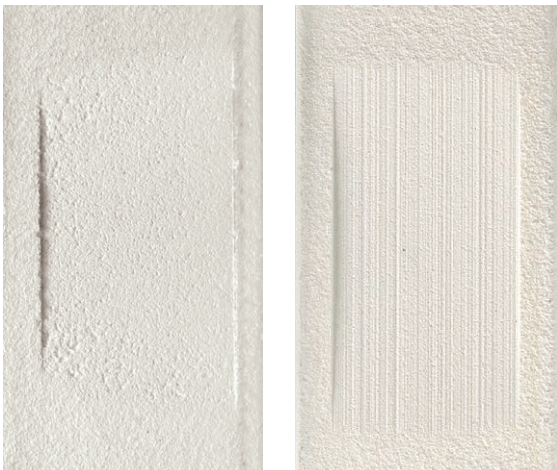
Examples of cleanly cut ceramic abrasible coatings @ 1100 °C (2012 °F). Left: against an un-tipped blade, Right: against a cBN tipped blade
