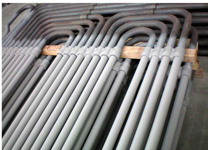
Thermal spray coated boiler tubes. Left: coated and ready for installation. Right: after one year in service.
