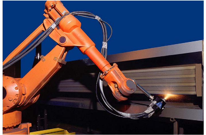
A Oerlikon Metco Smart Arc system robotically spraying a boiler waterwall section in shop.
