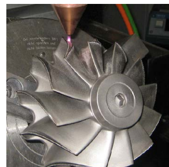
3D turbocharger blade tip repair with MetcoClad 625
