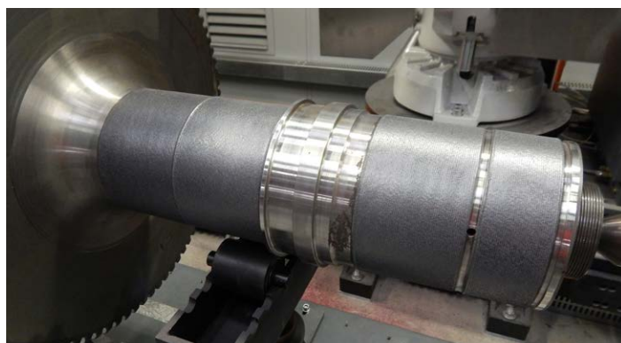
Repair of shafts with iron-based alloys
